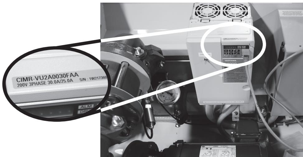
Figure 6 - A photo showing where the rated output current is printed on the VFD. The VFD shown here is rated for 30.0A/25.0A.
