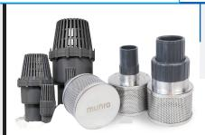
Designed specifically for irrigation, these foot valves are non-corrosive and offer a hard-to-clog, particulate strainer. Spring-loaded design through 3" or a flapper style through 10". Available in national pipe thread, PVC socket weld, or flanged (8" and 10" only).
