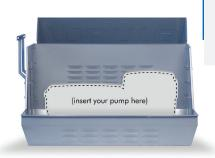
Power-coated stainless steel pump enclosure, includes two inlet and outlet options, ventilation louvers, mounting for a pump control panel and security features. Pump can position facing left or right.
