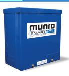
Using a pressure sensor and optional temperature sensor, the SmartBox protects the pump from run dry and overheating – avoiding costly pump meltdowns. This universal box works with any 3/4 - 5 hp lawn pump. Also available: a reduced incoming amp model for compatibility with 2-wire systems.
